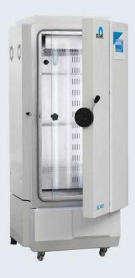
GC 401 Growth Chamber is developed for simulating real environmental conditions by controlling temperature, humidity and day-night lighting cycles. GC 401 can be used for different purposes by the help of state-of-art design:
